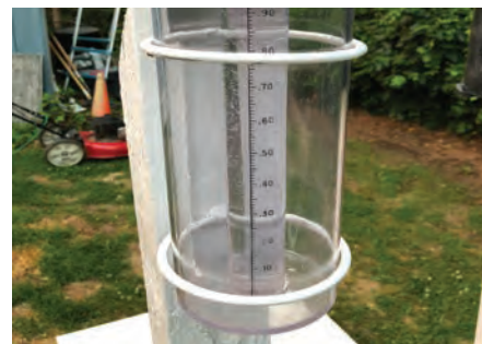
CoCoRaHS rain gauges are accurate within 1/100 of an inch. Courtesy photo
